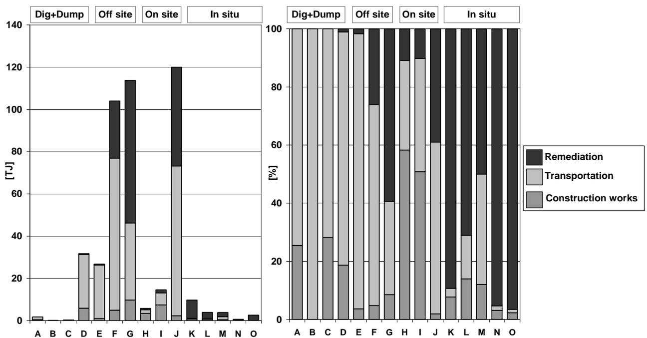
**FIGURE 2: The absolute and relative values of the remediation, transportation and construction in different projects A – O in the impact assessment category “Cumulative Energy Demand”**
