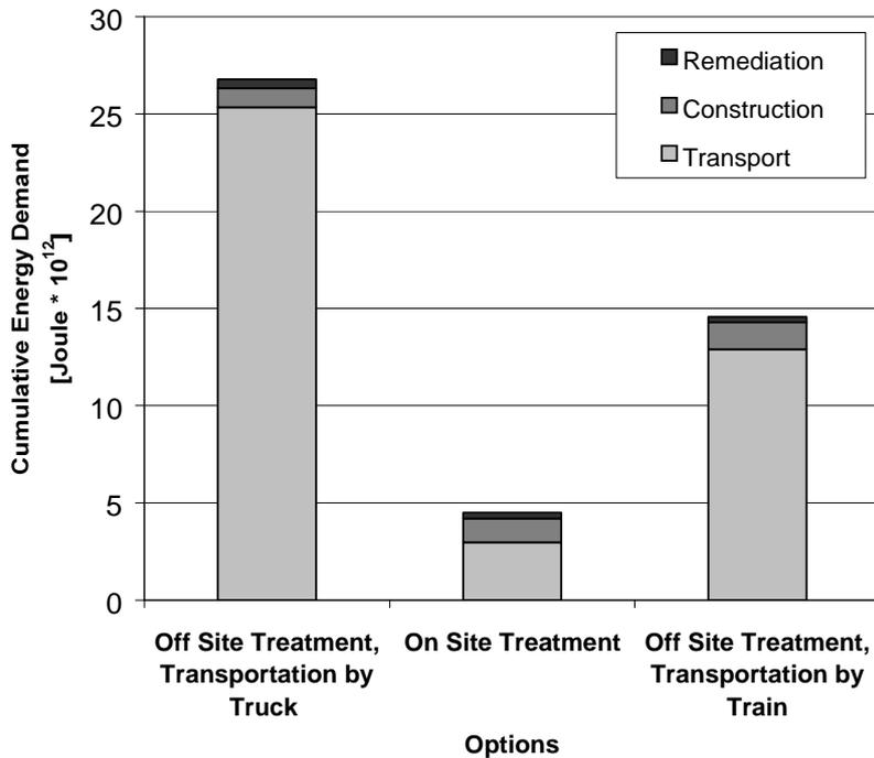
**FIGURE 5: The “Cumulative Energy Demand” for a project of biological treatment with different options of transportation**
